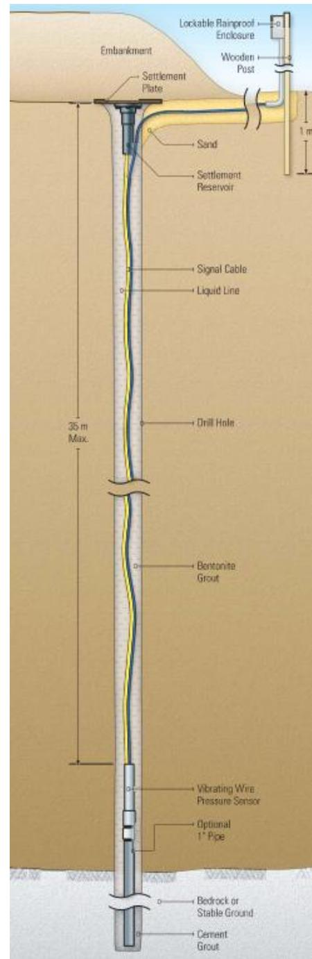
Figure 3, Subsurface Settlement System
