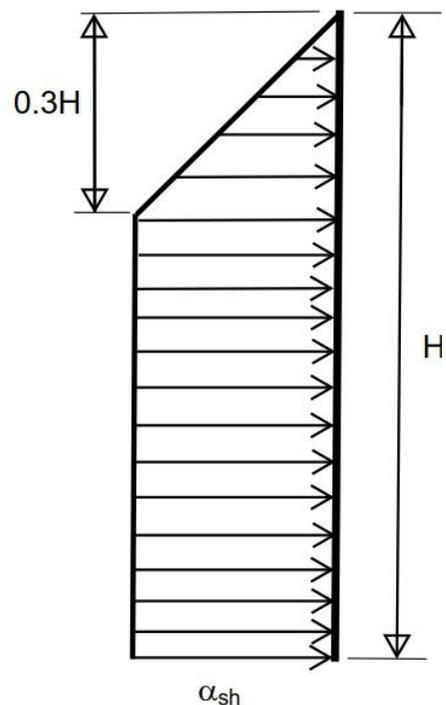
Figure 2, Abutment wall Loading Diagram
